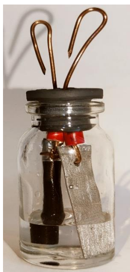
Figure (1) Illustration of an aluminum-graphite electrochemical cell
