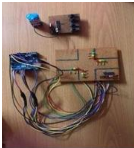
Fig. 7 Hardware of Traffic Signal Control System
