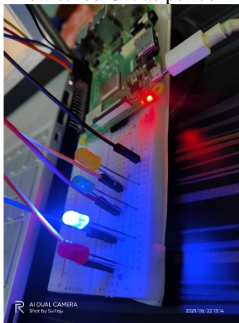
Fig3: LED-1 Switched OFF and LED-2 switched ON per command given.
