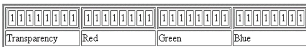
Figure 2: BIT Transferred for Red, Green and Blue plane (24bit=8bit red;8-bit green;8bit blue)
