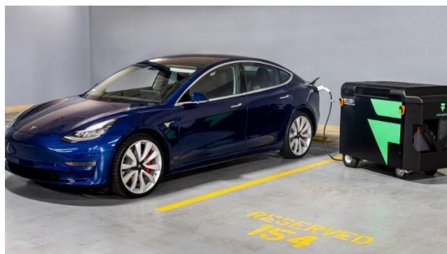
Fig.4 Mobile EV charging station
