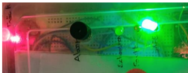
Fig. 16. Safe Indication at local BMU
