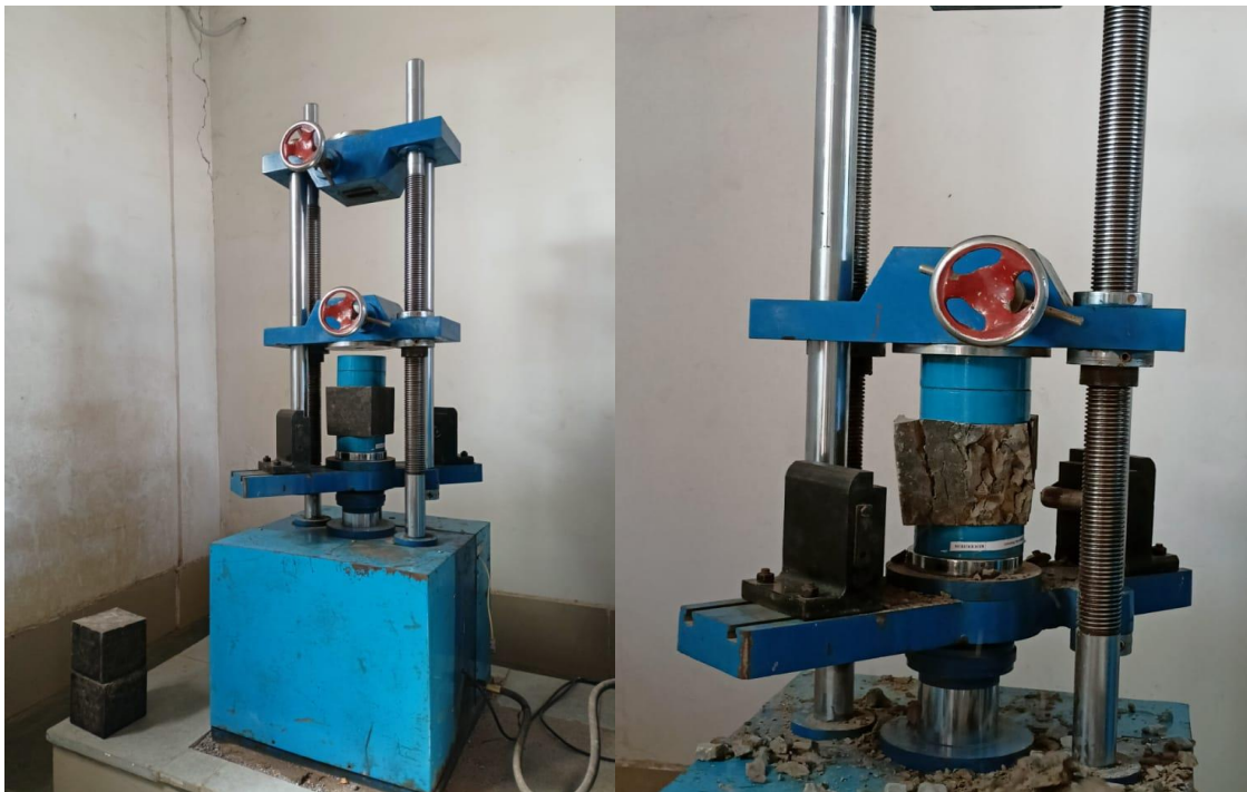
Fig 3.3 Before cracks & After cracks during CTM test
