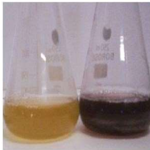
Silver nitrate (1 mmol l -1 ) in conical flasks before (left) and after (right) exposure to Phoma glom erata culture supernatant
